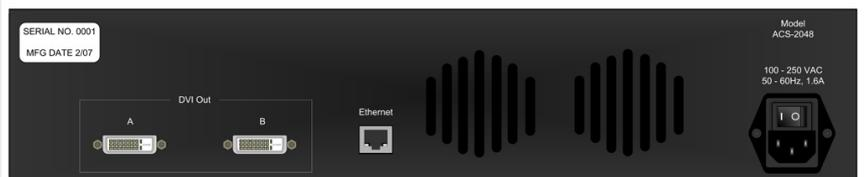
As the ideal peripheral for all digital cinema installations, the ACS-2048 is an 8x1 switcher that accepts "universal" input formats, and outputs 12-bit twin DVI at 2048 x 1080 - one of the digital cinema standards. With a high-quality scaler at its core, upconverting any input format is as simple as "auto-acquiring" and selecting the desired input.
