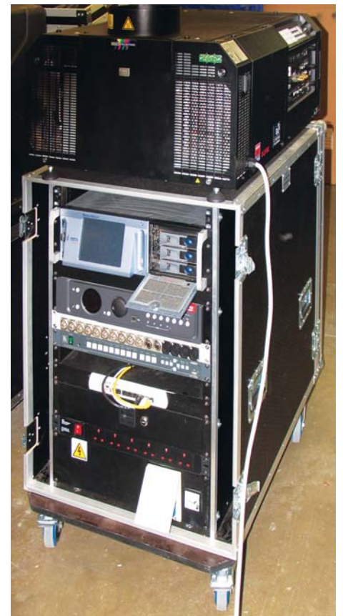
FP's portable Digital Cinema package complete with Doremi server and full cinema sound equipment, ready to be wheeled in to provide a 'pop-up' cinema anywhere, or as an emergency kit to rescue any show.
